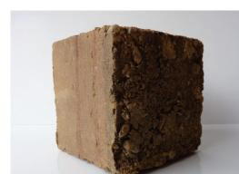
Rammed earth construction Rammed earth construction uses compressed soil as a building material. This technique generates an resource that is simply returned back
