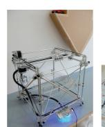
RepRap by Adrian Bowyer & RepRap community RepRap is a 3D desktop printer, capable of printing plastic objects. Since many parts of RepRap are made from plastic, and RepRap car print those too, it is a self-replicating machine - one that anyone can build given time and materials. www.reprap.org
