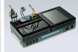
Buglabs offers a module-based Linux computer for rapid prototyping. It provides a collection of electronic modules that can easily be plugged together and programmed to make any device you want. www.buglabs.net
